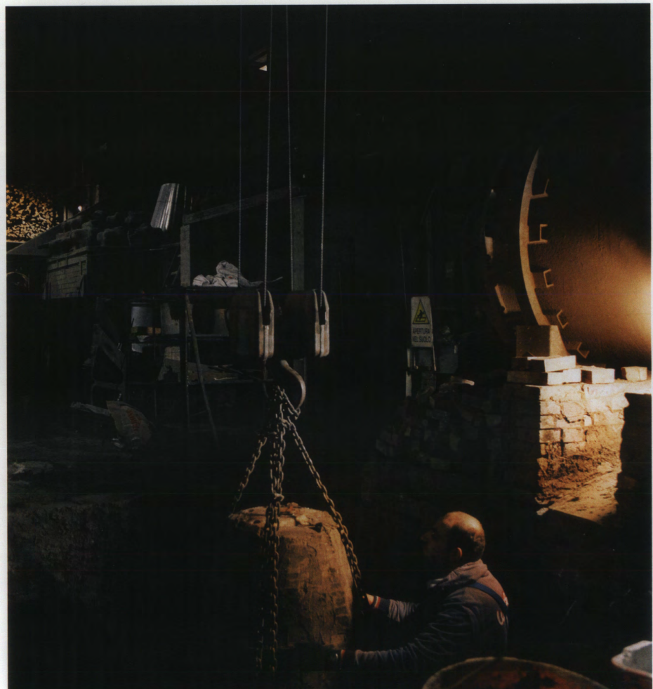
two works in progress await the next stage of production. Right: bell molds are lowered into this deep casting pit, ready for molten bronze to be poured over them. Once cooled, the bronze bell is lifted from the pit and hand finished by artisans who chisel and polish it before attaching the clapper and testing the chime
